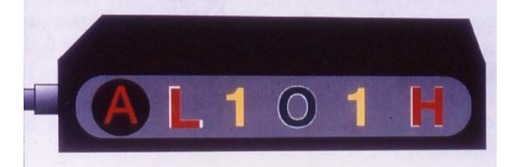
A "typical" primary display might look like this, indicating "A" for alarm, "L" for low ppO2, "H "for high ppO2, and "0" for the correct set-point.
