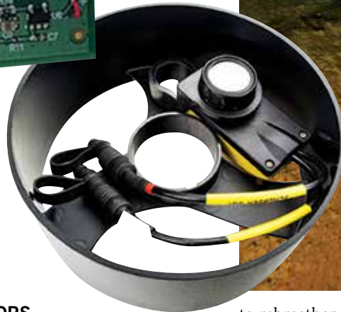
From far left: Hollis Explorer CO 2 sensor with humidity filter; Polestar Technology's sensor circuit board; AP Diving CO 2 sensor positioned in lid; a rebreather diver contemplates his gas mix
